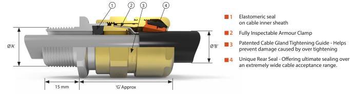
The 153/X Cable Gland is general purpose cable gland for use with wire braid, steel wire armour, elastomer and plastic insulated cables. The gland provides an elastomeric seal on the cable inner sheath, and a low smoke, zero halogen IP and retention seal onto the cable outer sheath.
